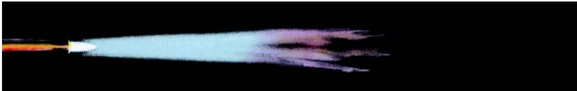
Oxidizing Flame (Acetylene and excess oxygen, 6300°F)
